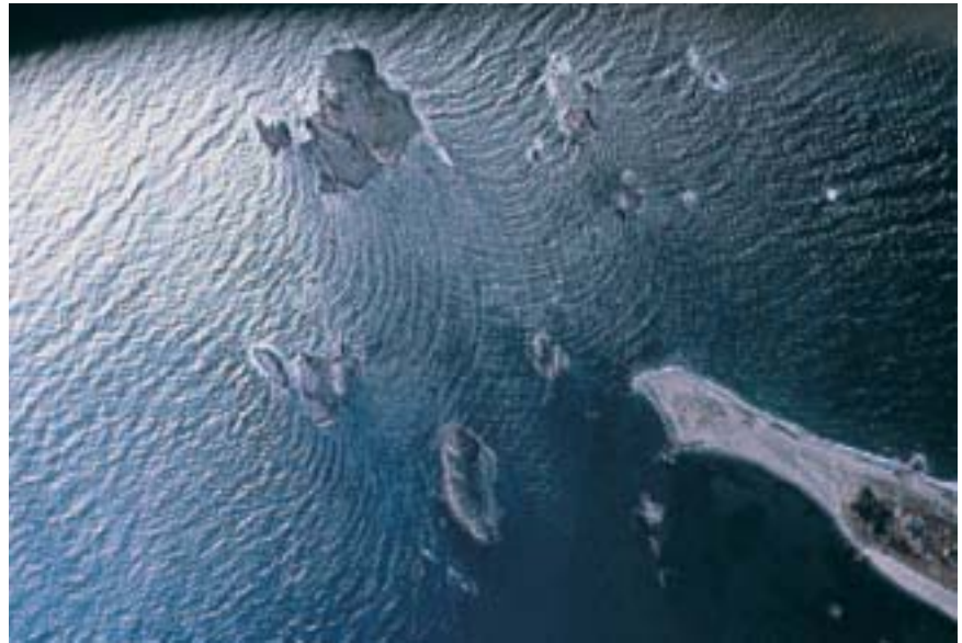
Figure 18 Diffraction causes ocean waves to change direction as they pass a group of islands.
