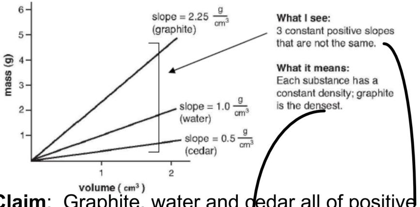
Claim: Graphite, water and dedar all of positive slopes but are not the same. Graphite has the highest slope and is the most dense, the water and cedar has the lowest slope.
